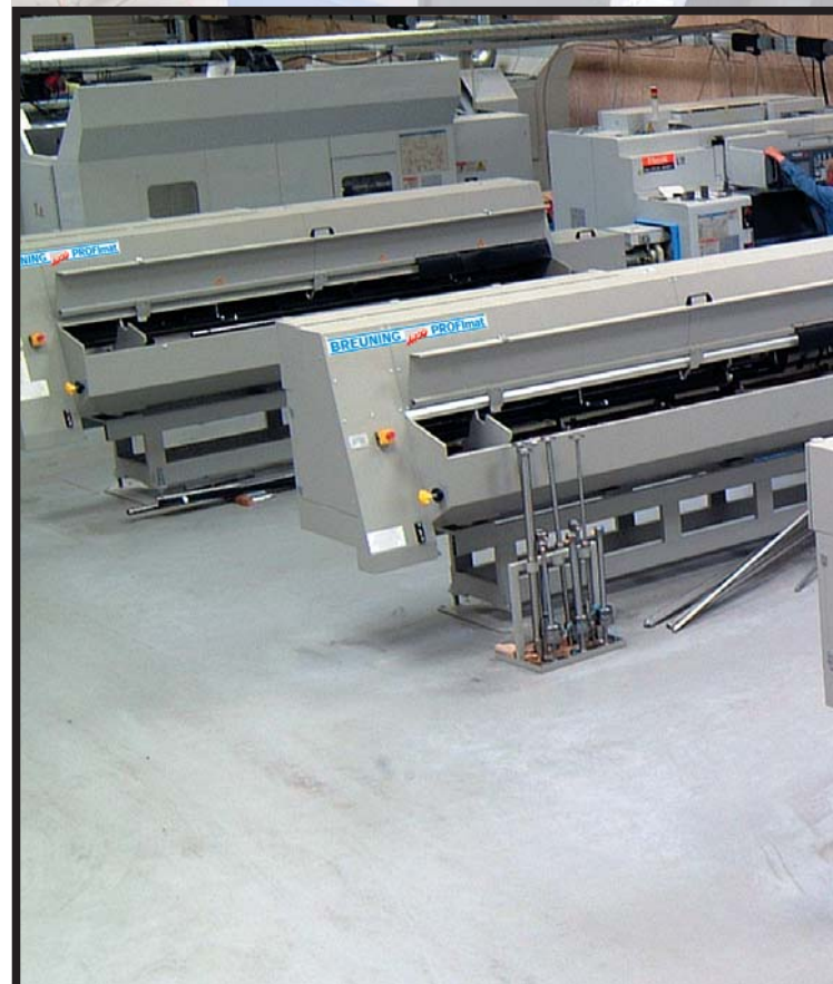
BREUNING PROFimat multi-channel loading magazines
