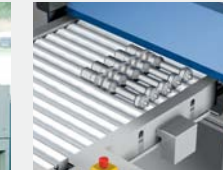
ILS-TEX Transfer of the individual parts to the integrated indexed conveyor
