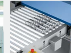
ILS-TEX Transfer of the individual parts to the integrated indexed conveyor
