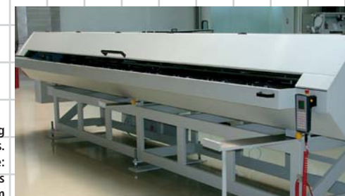
ILS-SB-TBL for 6 m long extruded sections. In figure: Material diameters to 130 mm
