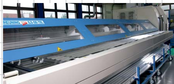
ILS-SB-TBL for 6 m long extruded sections. In figure: Material diameters to 130 mm
