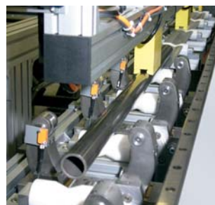
Steady rest guiding system LF In figure: Open steady rests and integrated loading gantry with magnetic holder
